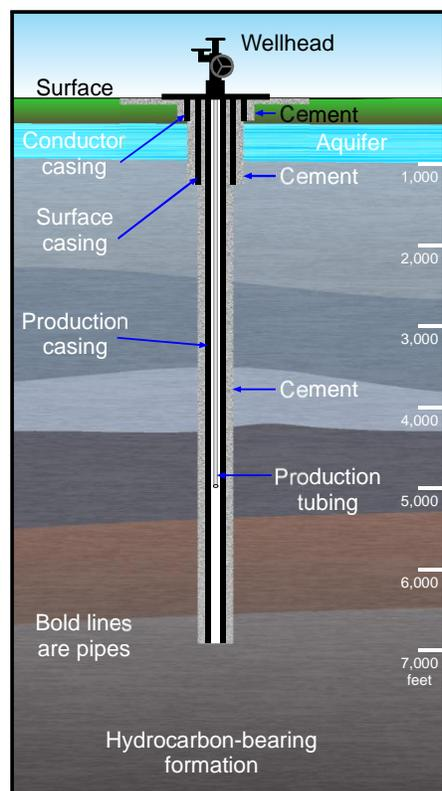
**FIGURE 8. WELL CONSTRUCTION**
