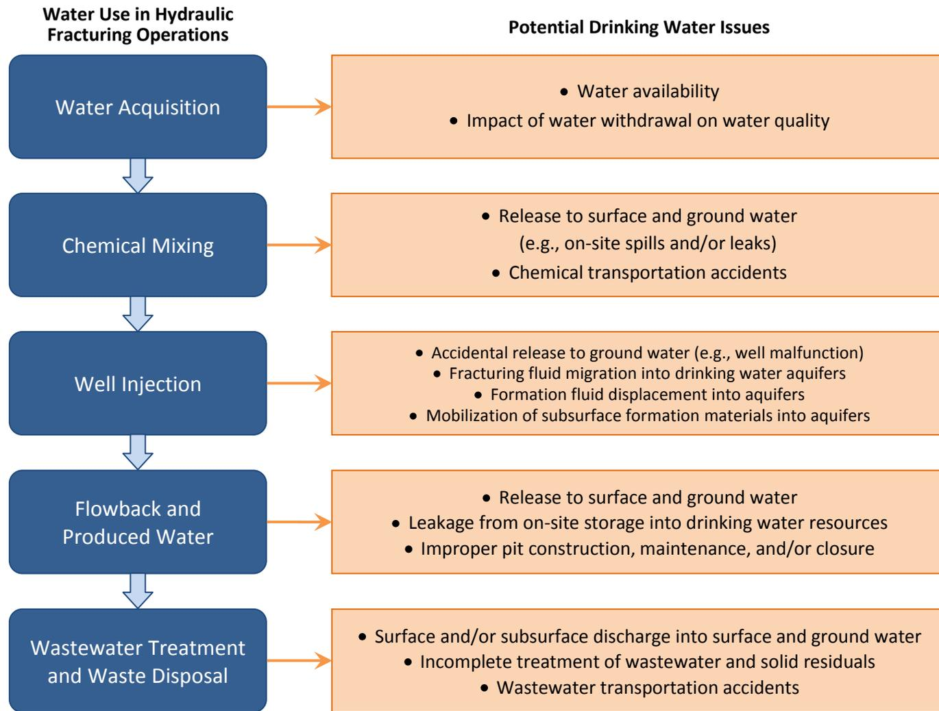
FIGURE 7. WATER USE IN HYDRAULIC FRACTURING OPERATIONS
